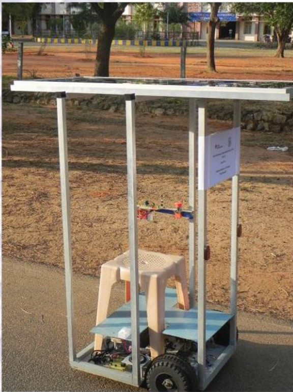
Solar Powered Wheelchair developed by P.Kishore and Team
